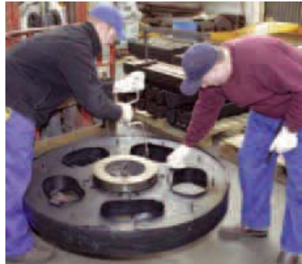
■ ABOVE : LEADING HAND GRANT VAILE (LEFT), WITH A GRINDING WHEEL FOR M.I.M. HOLDINGS, A MAJOR AUSTRALIAN MINING COMPANY, MANUFACTURED AT SKELLERUP'S LARGE PRESS FACILITY.
