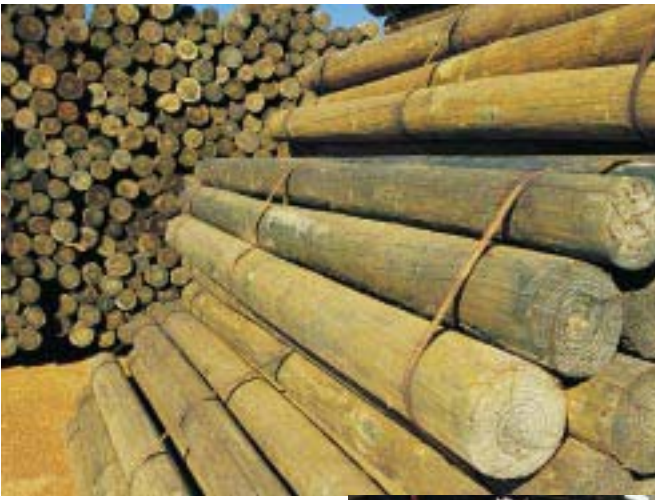
Above Treated pine rounds stacked at Sotico's Mundijong treatment plant. Timber is preserved using a copper, chrome and arsenic (CCA) treatment process.
