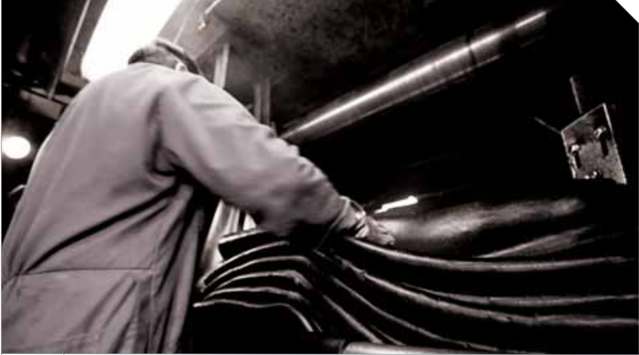
+Above Rubber being extracted from the mill after mixing in the Primary Process Department.
